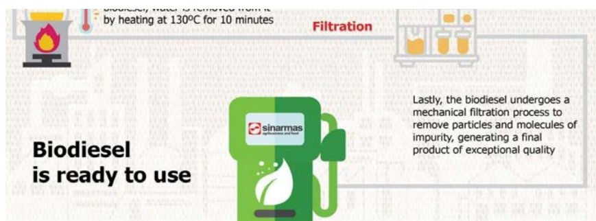
Figure 120: Biodiesel is produced via transesterification, where oils react with alcohol in the presence of a catalyst, followed by refining, washing, drying, and filtration to obtain fuel-grade biodiesel 162 .
