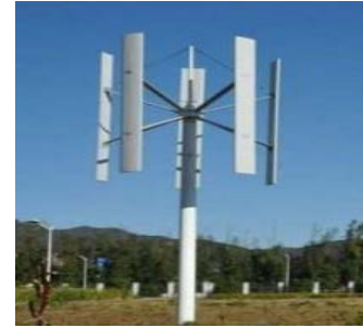
Figure 67: Vertical axis wind turbines can capture wind from any direction and are suitable for urban or small-scale applications.
