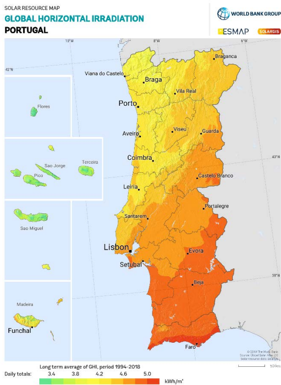
Figure 31: Southern Portugal receives the highest solar irradiation, making it ideal for large-scale solar power projects
