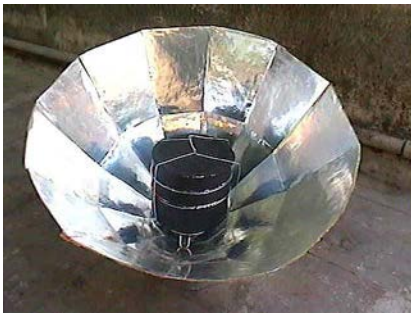
Figure 40: Solar furnaces use parabolic reflectors to focus sunlight for cooking and heating.
